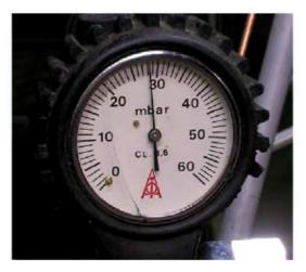
Turn the adjustment screw with a screwdriver so that the pressure gauge reading corresponds to the pressure applied.
