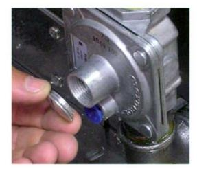
• Remove the screw of protection of regulator setting with a screwdriver.
