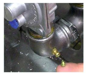
· Remove the screw closure of the pressure tap with a screwdriver.
